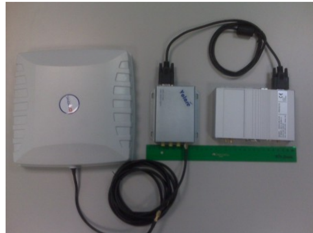
Antenna, Reader and Movilcom Plus
